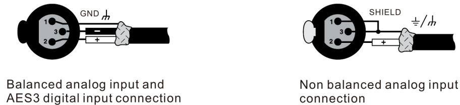
Figure 3. Balanced and unbalanced XLR input wiring
