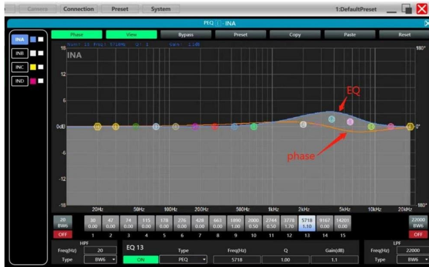
Figure 61. IIR equalization changes both magnitude and phase
